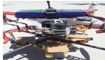
Figure 5: A prototype of quadrotor that shows the positions for ultrasonic sensors.
