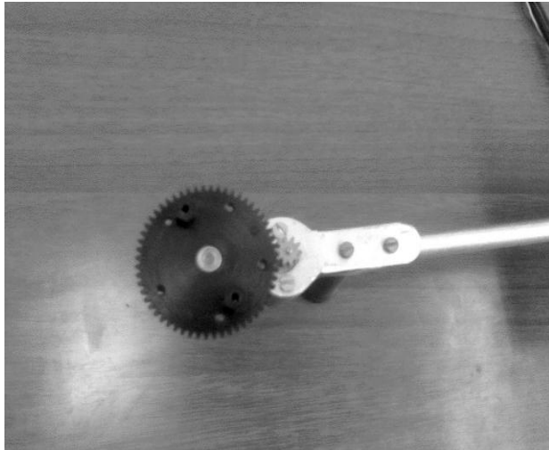
Figure 5. Gearbox and Motor Mount.
