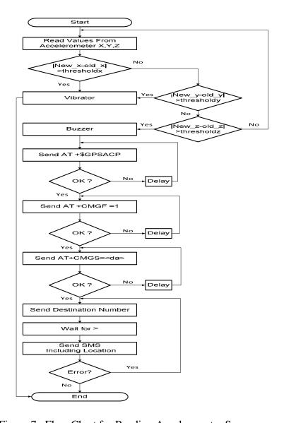
Figure 7. Flow Chart for Reading Accelerometer Sensor.
