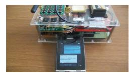
Figure 9: Testing GSM-GPS Module and Accelerometer Sensor.
