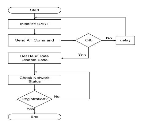
Figure 3. Flow Chart for Module Startup
